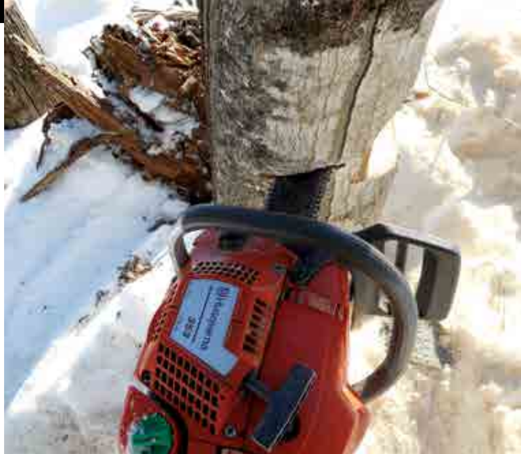
The open-faced notch (right) with a bore cut behind it. Be sure to bore well behind the notch—I bored too close to the notch, the hinge crushed and my saw was pinched. I used a second saw to make a new cut 16 inches above this one.
