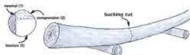
FIGURE 2 Bucking when the log is unsupported on one end. First, cut an inch or so into the bottom side so the wood will not tear when the cut breaks. Then, cut through the top, off side first. On sloping ground, work uphill of the cut so the log does not roll on you.
